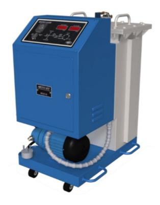
Fine suspended particles contained in oil entering in the oil cleaner from oil inlet provided at the bottom, gets ionized & statically charged while passing through electrostatic field generated by applying High voltage (6kv/12kv) across +ve/-ve electrodes. According to the nature of the charge, such charged particles get attracted towards either of the electrodes.
